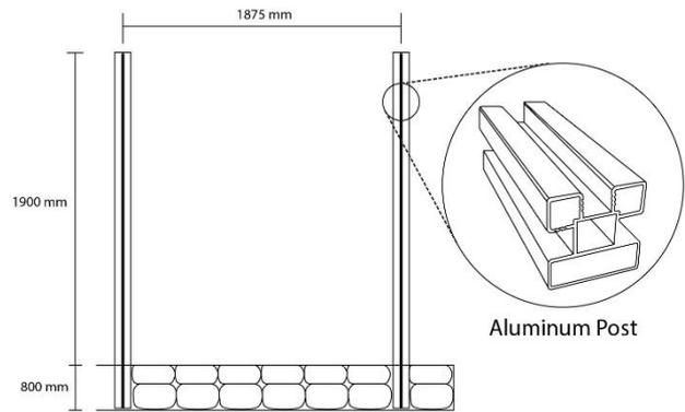
**Step 1.** Mark out fence line and dig holes at 1875mm centres. 350mm wide by 800mm deep (1000mm in sand)
