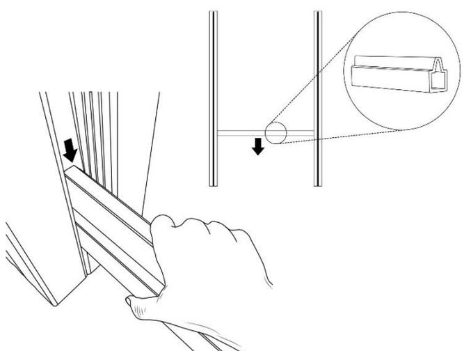
**Step 3.** When concrete is hard, slide spacer down the grooves in the slots in the post and screw using the 8g x 50mm self drilling screw so the TOP of the spacer is at 1880mm from the top of the post. The bottom rail sits on this so ensure all spacers are the same so the rail sits level.
