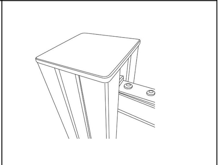
**Step 8.** Install post cap. You may need a rubber hammer to lightly tap into place.
