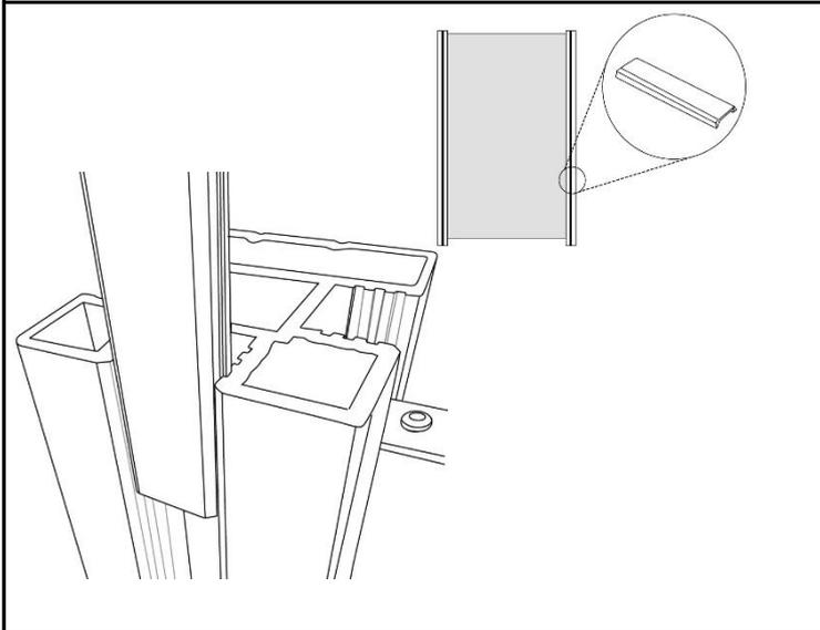
**Step 7.** Slide the slot cover down the grooves in the post of the unused slot and trim with a hacksaw.
