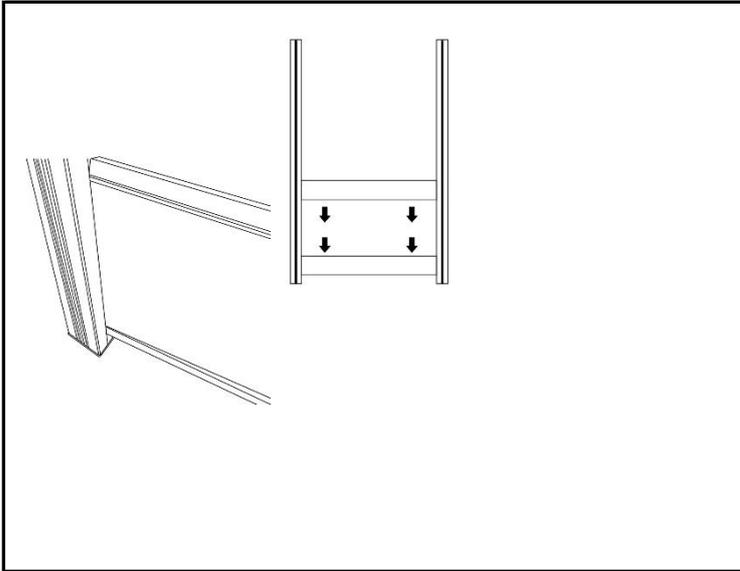
**Step 5.** Place boards in slot on the posts and rest on the bottom rail. Repeat for all boards in the bay.
