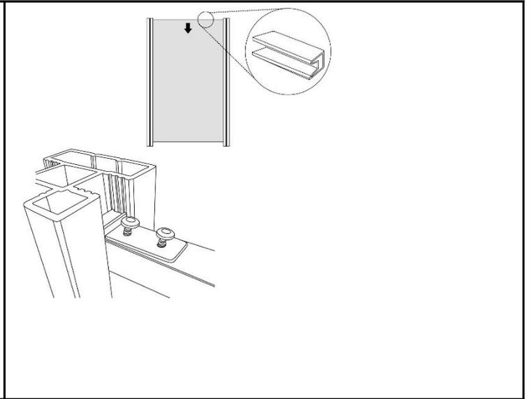
**Step 6.** Place the top rail on the last board and put the L clip in the grooves in the post slot. Secure to the top rail rail using 2 of the 8g x 25mm self drilling screws. Repeat at other side.
