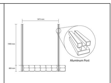
**Step 2.** Pour concrete ensuring the posts are set straight and square. Ensure they are at 1875mm centres apart and the top of the post at 1900mm from the FINISHED ground level. Clean any concrete splatters of the posts while still wet with a soft brush.
