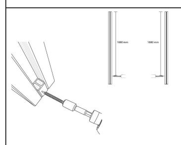
**Step 3.** When concrete is hard, slide spacer down the grooves in the slots in the post and screw using the 8g x 50mm self drilling screw so the TOP of the spacer is at 1880mm from the top of the post. The bottom rail sits on this so ensure all spacers are the same so the rail sits level.
