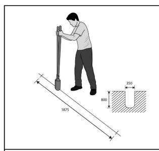
**Step 1.** Mark out fence line and dig holes at 1875mm centres. 350mm wide by 800mm deep (1000mm in sand)
