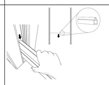
**Step 4.** Set the bottom rail on the spacers in the post with the tongue facing up. Check again the rail is level and at the same height as the rail on the next bay. There should be a 4mm gap at either end of the rail to allow for heat expansion.
